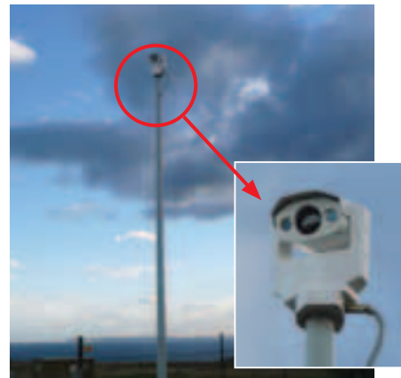
The FLIR Systems PTZ-35x140 MS. It contains 2 thermal imaging cameras and one daylight/lowlight camera.
